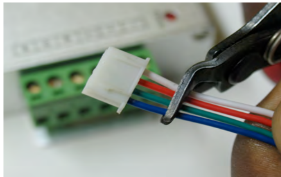
Cut one side of connector and wire to leads
